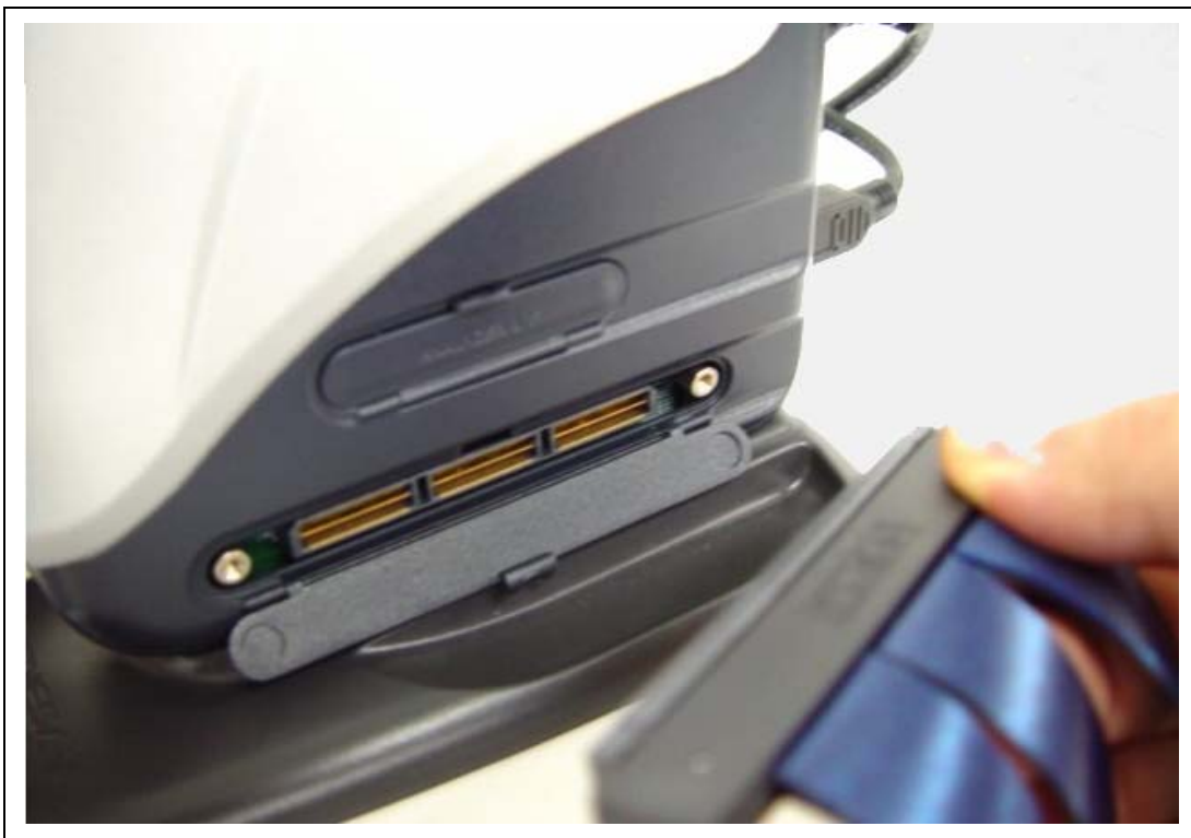
Figure 2.7 Connecting the Trace Cable to E200F
